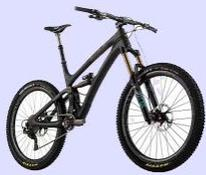
Carbon XTR Complete Mountain Bike. Carbon fiber frame, FOX Float X CTD rear shock & 36 160 Factory fork, 44/56mm Chris King tapered headset, SHIMANO: XTR 11-speed shifters; XTR 11-speed read derailleur; 32 t XTR crankset; PF92 bottom bracket; 11-40 t XTR cassette; XTR 11-speed chain;
